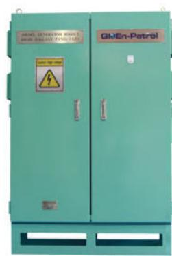
The major function of Power Supply Panel is to operate the medium pressure UV lamps UV. It controls the strength of UV lamps with the capacitors mounted in the Panel. Also it detects whether the UV lamps are functioning properly or not. The temperature sensor is mounted inside to monitor temperature in order to give an alarm to an operator and shut down the system in case of overheating.
