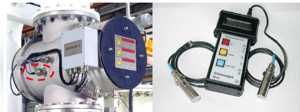
Figure 7.39 UV intensity housing (Left) and UV reference radiometer (Right)
